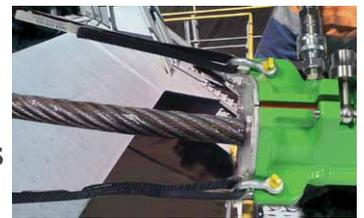
WRL Penetrating Grease VPG-0, is a soft, semifluid formulation designed to coat wire rope with a thin lubricant film as well as penetrate to the core. Its tacky, water-resistant characteristics enable it to adhere strongly and to seal out damaging moisture. Viper WRL Penetrating Grease contains a wear-reducing additive that protects against premature wear and shields metal against corrosive attack.
