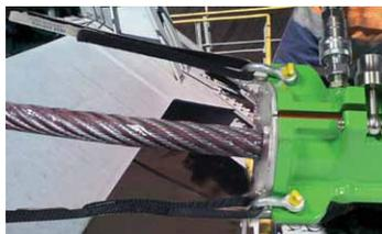
WRL Coating Grease VCG-1, is a technologically advanced lubricant designed to withstand water washout, protect against corrosion, penetrate and also provide extreme pressure protection for winch drums and sheaves. The red tacky NLGI#1 grease will provide superior service life in marine and mining applications with non drip or fling tendencies.
