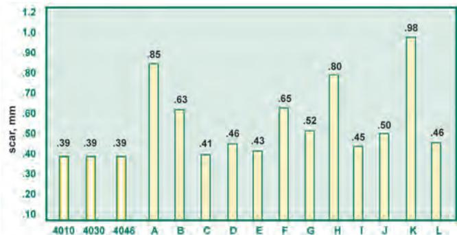
The four ball wear test is used to determine the relative wear preventative properties of lubricating fluids. Lubricants are compared based on the average size of the scar diameters worn in the three lower balls after rotation of the upper fourth ball in the test procedure. A smaller wear scar size indicates the lubricant is providing better wear protection. **QUINPLEX OILS HAVE THE SMALLEST SCAR AND BEST WEAR PROTECTION OF ALL OILS TESTED!**
