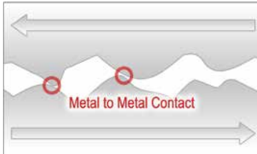
Figure 1: Asperities on touching metal surfaces
